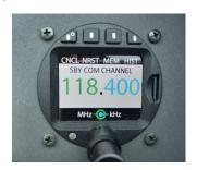
Volume – just 'turn' the inner knob, without the need to go to CHN screen
