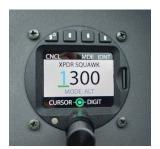
To change squark code – XPDR – use the outer knob to change the position in the squark code -rotate the inner knob to change the numbers, then enter (inner)
