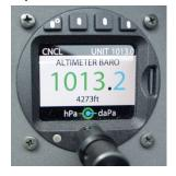
To set the altitude before launch – BARO – Rotating the outer and inner knobs alters the barometer which is linked to the altimeter. Adjust to the airfield altitude. Push the inner knob to enter. Do this as part of every pre-flight check.
